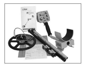
Assembling the Tejón is simple and requires no special tools. Just install the battery packs, mount the searchcoil on the lower pole assembly, connect the pole assemblies together, wrap the excess cable around the pole, and plug the cable into the control housing. Finally, adjust the pole length and searchcoil angle and you're ready!
