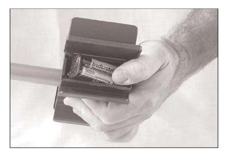
When returning the holder, note the position of the spring clips inside the armrest housing and make sure that the battery pack contacts fit snugly against the springs. Insert the side with the contacts first and then press down on the left edge of the battery holder to reseat the holder.
